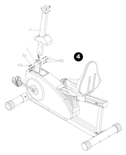
**4.** Slide the console tube (2) through the console tube collar (14). Connect the computer cable in the console tube (2) to the computer cable in the main frame. Attach the console tube (2) to the frame (1) with the locknuts (49), flat washers (50) and screws (56) provided. Attach the console tube collar (14) to the main frame (1) with screws (57).
